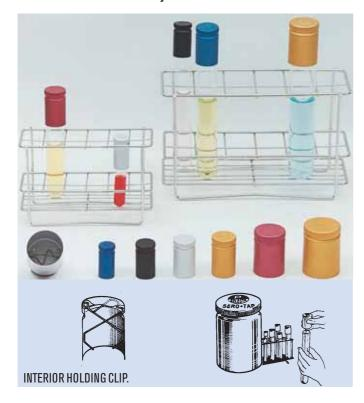
Made of anodised aluminium with internal AISI 304 stainless steel spring inside the cap. Not hermetically sealed. Autoclavable at 1 bar.
